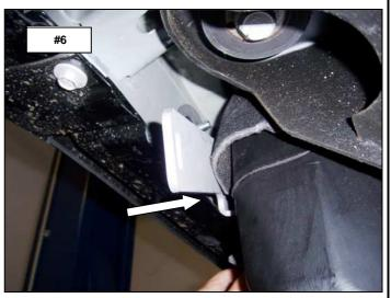
**Step-4** Position the obround hole in the front of the bracket over the T-Bolt and install (1) 3/8" flat washer, (1) 3/8" lock washer and (1) 3/8" hex nut. Position the flange of the bracket on the bottom of the pinch mold and align the obround hole with the U-Nut and install (1) 5/16" flat washer, (1) 5/16" lock washer and (1) 5/16" x 1" hex bolt. Leave the nut and bolt loose for final adjustment. **Photo #7 & #8**
