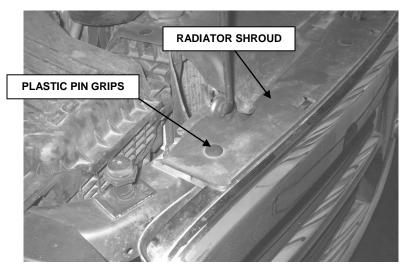
STEP 4. OPEN THE HOOD AND REMOVE THE PLASTIC PIN GRIPS AND RADIATOR SHROUD.
