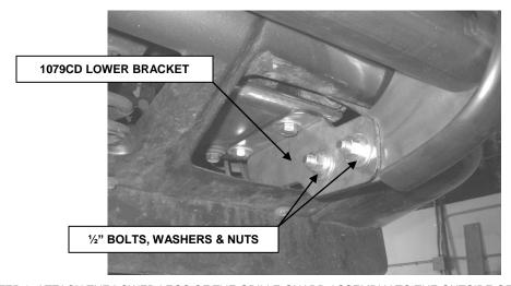
**STEP 8.** ATTACH THE LOWER LEGS OF THE GRILLE GUARD ASSEMBLY TO THE OUTSIDE OF THE LOWER MOUNTING BRACKETS USING THE  $1/2^{\circ}$  X 1  $1/2^{\circ}$  HEX BOLTS, WASHERS, AND NUTS.
