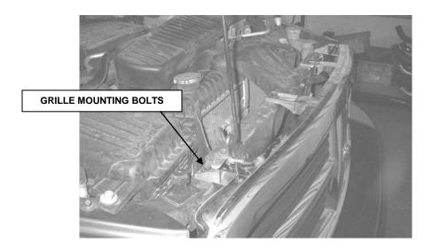
STEP 5. REMOVE THE (4) BOLTS SECURING THE TOP, AND UNSNAP THE ENDS OF THE GRILLE.
