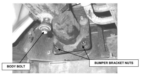
**STEP 1.** BEGINNING WITH THE DRIVER SIDE, LOCATE AND REMOVE THE BODY MOUNTING BOLT FROM THE BOTTOM OF THE FRAME, AND THE HEX NUTS THAT SECURE THE BUMPER BRACKET TO THE FRAME.
