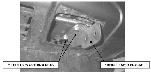
STEP 3. ATTACH 1079CD LOWER BRACKET TO THE BOTTOM OF 1079BD USING THE  $\frac{1}{2}$ " X 1  $\frac{1}{2}$ " BOLTS WASHERS AND NUTS AS SHOWN. REPEAT THE ABOVE STEPS FOR THE PASSENGER SIDE LOWER MOUNTING BRACKET.
