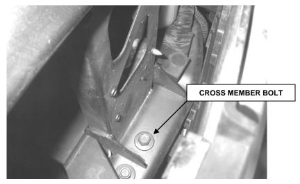
**STEP 6.** REMOVE THE CROSS MEMBER BOLT. ACCESS THE BOLT BY PULLING OUTWARD ON THE TOP OF THE GRILLE.
