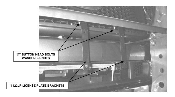
**STEP 12.** IF YOUR STATE LAW REQUIRES A FRONT LICENSE PLATE, ATTACH THE 1122LP BRACKETS, AND LICENSE PLATE TO THE GRILLE GUARD CENTER PLATE USING THE  $\frac{1}{4}$ " BUTTON HEAD BOLTS, WASHERS, AND NUTS.
